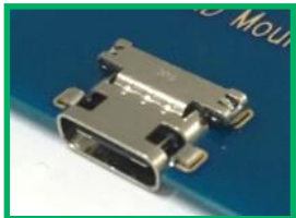
USB Type-C connector USB3.1 Gen1 Mid-mount Space saving
