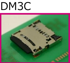
DM3C Push-Pull Type Top mount Height: 1.55mm Card Detection Switch
