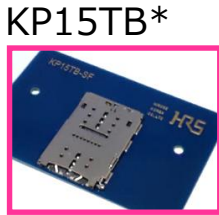
KP15TB* Tray Type Top mount Height: 1.37/1.55mm Card Detection Switch
