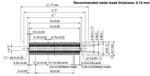
Note  $\square$  Cross-hatched portions, totaling n places, indicate the ground circuits.
