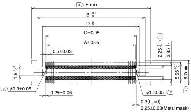
Note 1) The cross-hatched area 🖾 inside the SMT land may come into contact with the connector contacts and thus care should be taken that the pattern does not extend beyond the SMT land width.
