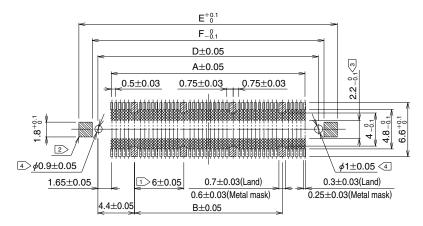
Note  $\boxed{1}$  Cross-hatched portions, totaling n places, indicate the ground circuits.
