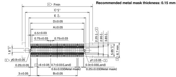
Note 1>Cross-hatched portions, totaling n places, indicate the ground circuits.
