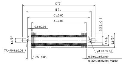
Note 1) The cross-hatched area 2 inside the SMT land may come into contact with the connector contacts and thus care should be taken that the pattern does not extend beyond the SMT land width.
