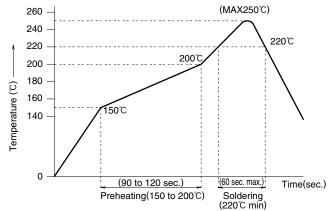
Note : The temperature profile indicates the maximum temperature of the connector surfaces at the highest point from the PCB mounting surface.
