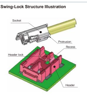
The protrusion on the bottom side of the socket fits into a corresponding recess on the header. This aligns the socket into the correct mating position.
