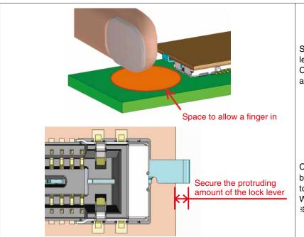
Space is required to operate the lock lever.
