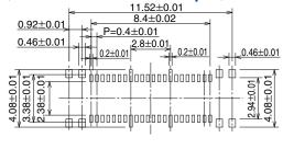
\*1: Caution! To insure proper lock lever operation, the FPC needs to be within the dimensions specified.
