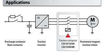
CA Series contactors are designed for load-free switching of traction motors of electric multiple units. In the event of a system fault, e.g. a short circuit in the traction inverter, the traction motors are instantly and reliably switched off, irrespective of the operating situation of the motor.
