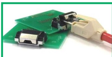
Foldable Open-Close RJ-45 Modular Jack Supports CAT5 Electrical Performance
