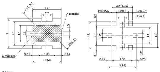
: This area must be free of conductive traces and solder resist on top layer.
