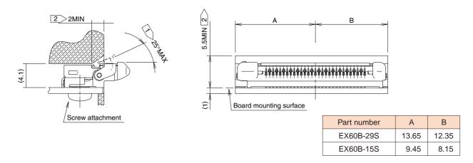
Notes The maximum opening angle of the rotating mating/unmating guide is 25°. Do not exceed this angle.
